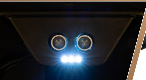
Backup sensor with LED lights
